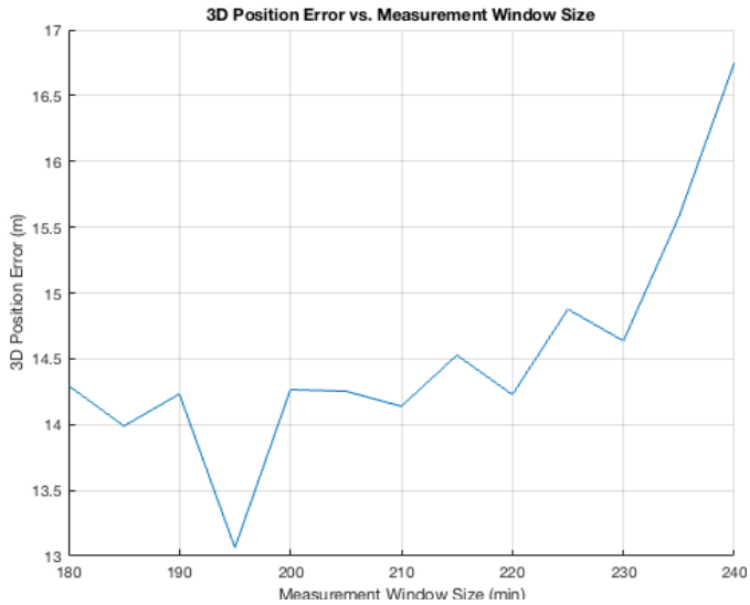
Figure 9: 3D Position Error vs. Measurement Window Size for LOC with 180 measurements per window and no surface constraint
