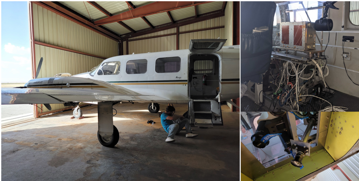
Figure 16. Images of the fixed wing testing setup with the Navigation Pod attached.
