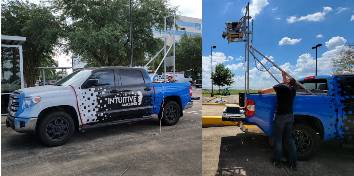
Figure 11. Images of the truck testing setup with the Navigation Pod attached.
