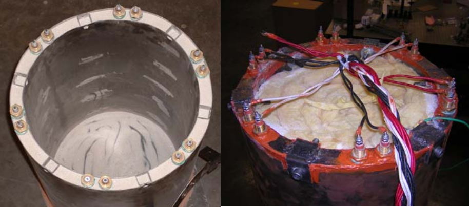
Figure 8. SMMRTG Casing with heater coils, MgO sand, and fibrous insulation
