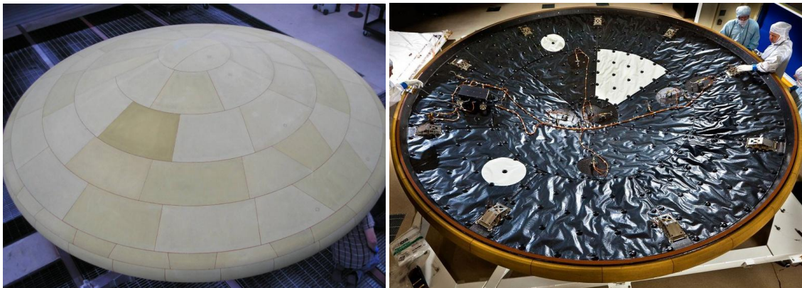
Figure 1. Completed MSL heatshield and underside with MEDLI system installed.
