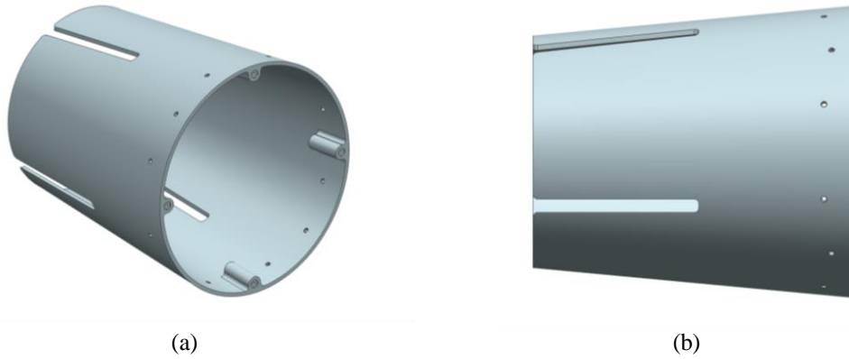
Figure 9. Backshell CAD views: (a) front isometric, and (b) side.
