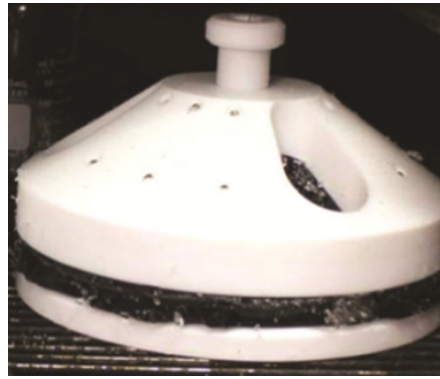
Figure 1. Open mold used in state-of-the-art processing of conformal ablators (Credit: Ref. 5).
