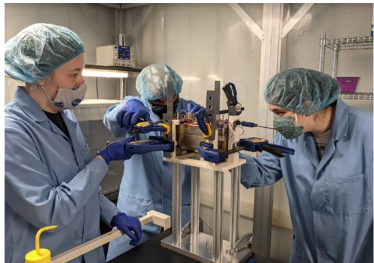
Figure 6: The Tank Manifold Mounting Process with the GSE Fixture
