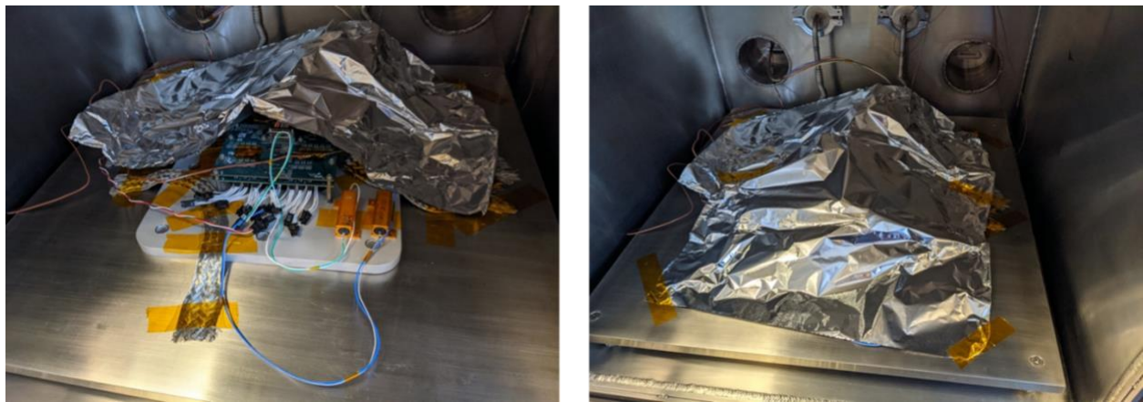
Figure 17. Flight controller with thermal straps and aluminum foil (left), and Flight controller completely covered with aluminum foil (right)
