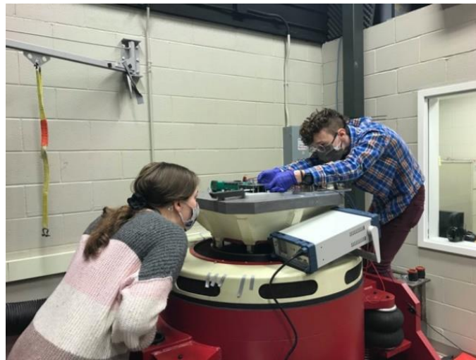
Figure 15. Short functional test during flight acceptance random vibration testing
