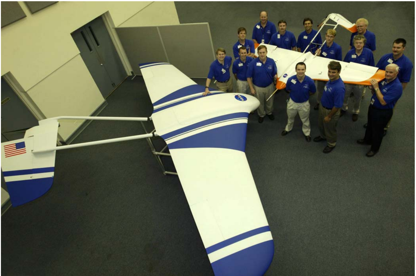
Figure 12: Mars airplane half- and full-scale flight test vehicles. The half-scale vehicle (orange) has the same general layout, folding scheme and airfoil characteristics of the Mars flight system. In addition to aerodynamics, the full-scale vehicle (blue) was designed with a flight-like composite structure, capable of withstanding launch loads.
