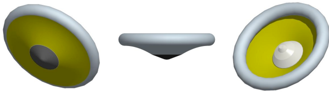
Figure 1. Tension cone inflatable aerodynamic decelerator.
