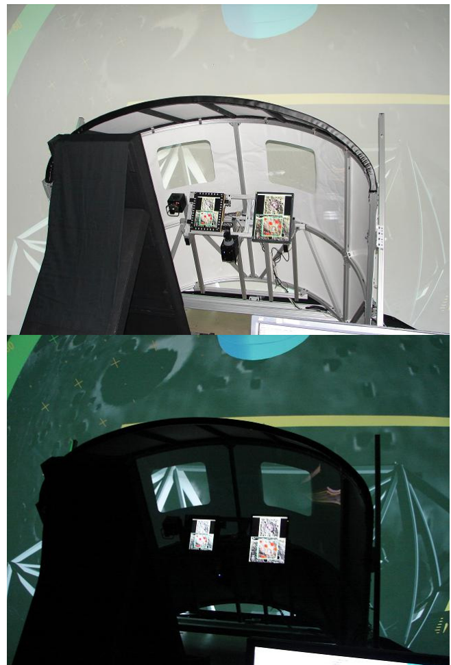
Figure 15: New lander mockup inside SES dome. The new vehicle “shell” with monitors showing ALHAT displays inside the cockpit. Outside on the dome a 3-D scene is rendered, and a person inside the “shell” would only be able to see it through the windows.
