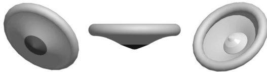
Fig. 2. Tension cone attached to an entry vehicle.
