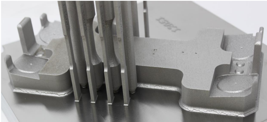
Figure 16. Manifold Reprint I – Crack Propagation (Credit: Volunteer Aerospace)
