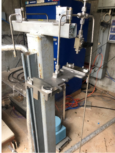
Figure 31. Manifold Burst Pressure Test
