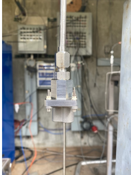
Figure 28. Recirculation Block Burst Pressure Test
