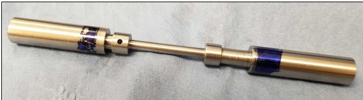
Figure 8: Finished torque rod core
