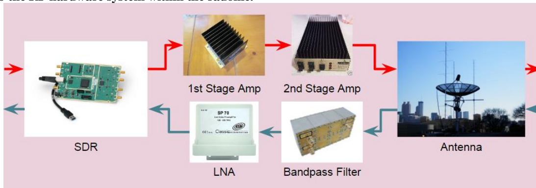
Figure 6: Flow of RF signals between the SDR and the antenna at the VL/MK stations. Red arrow indicates the uplink path and the cyan arrow indicates the downlink path.
