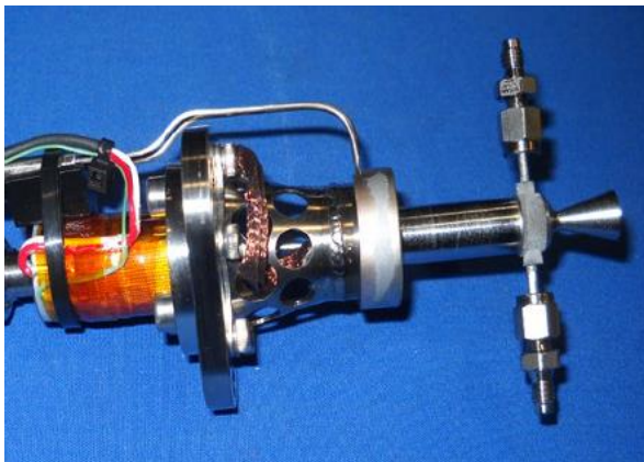
Figure 20: 1 N thruster in preparation for testing. Image courtesy of Tomas Hasanof.
