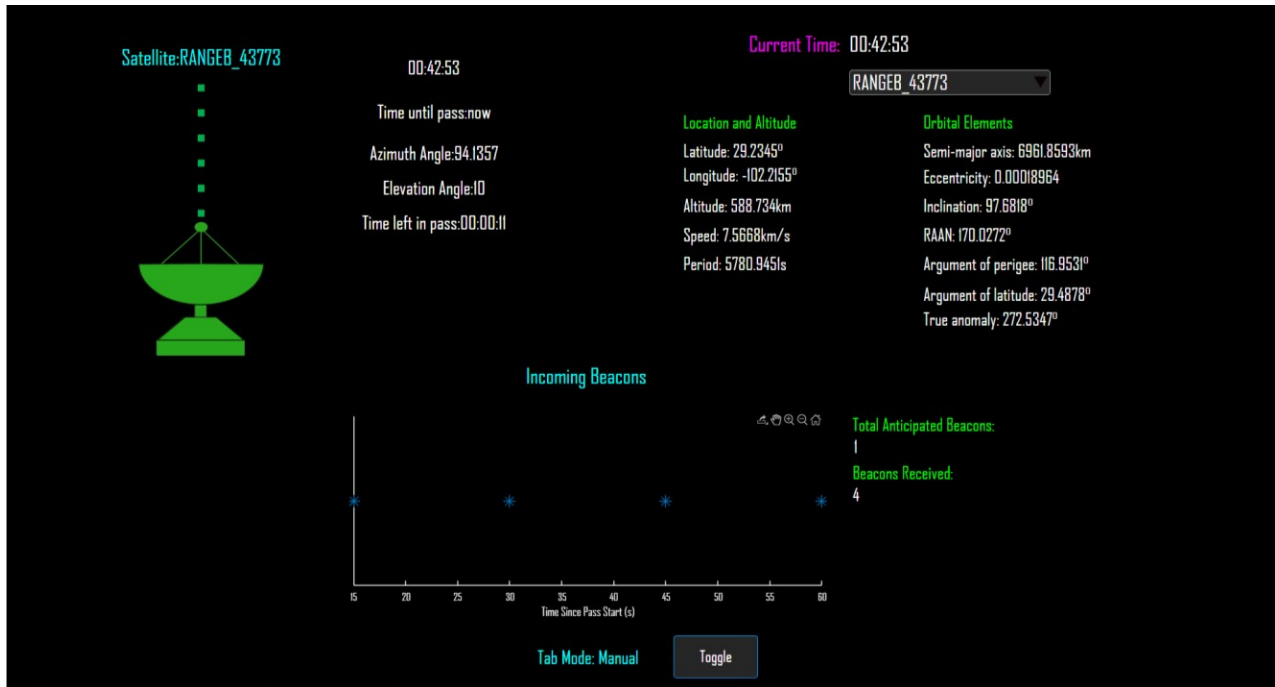
Figure 10. During pass display main screen when pass has started.
