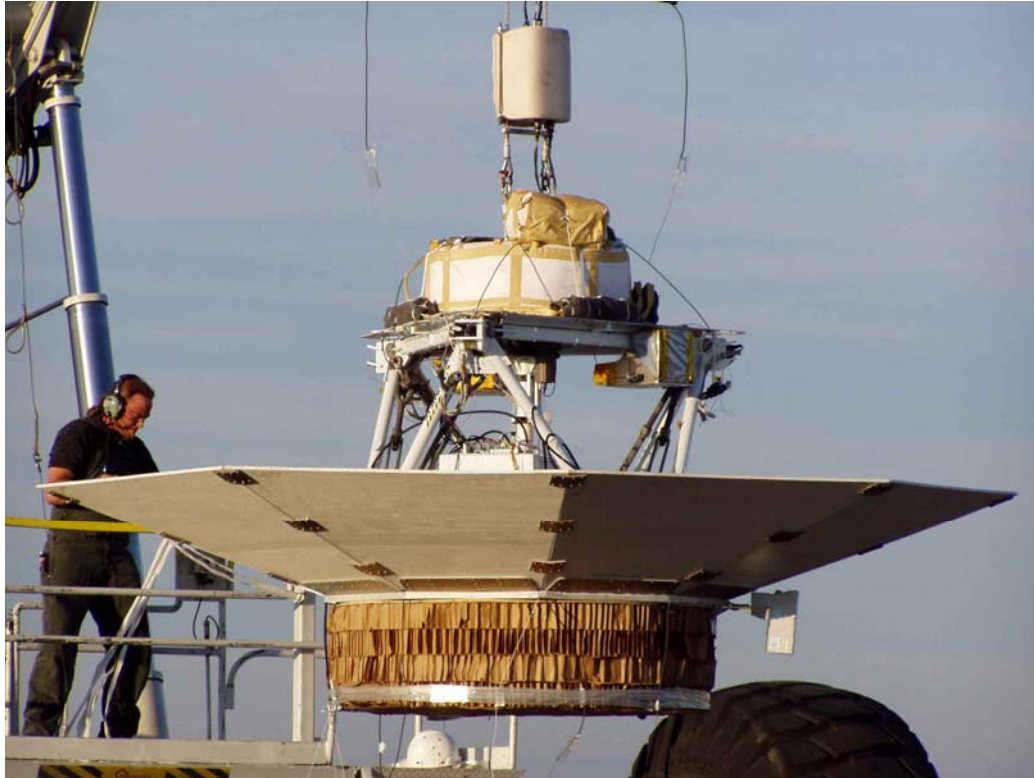
Figure 29: Mars Subsonic Parachute Test Gondola with Stowed Main and Drogue Chutes. 12
