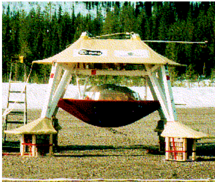
Figure 28: Huygens Drop Test Probe with Gondola. 9
