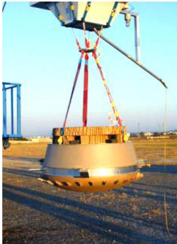
Figure 26: Huygens HASI Drop Probe (gondola, ring, cone, and upper cover). 3
