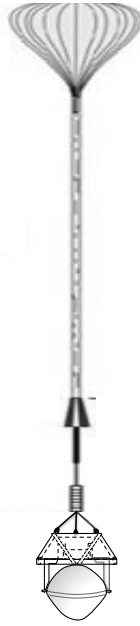
Figure 19: Concept for SPORE Drop Test Ascent Train (Not to Scale).
