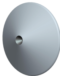
Figure 2. Example of a Central Retropropulsion Configuration with a Single Nozzle
