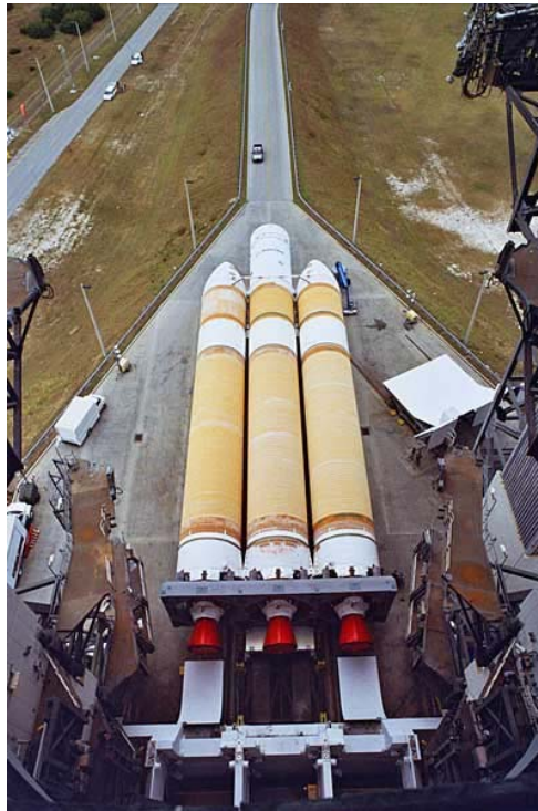
Figure 31: Delta IV Heavy Preparing to be Loaded Vertically onto the Launch Pad.
