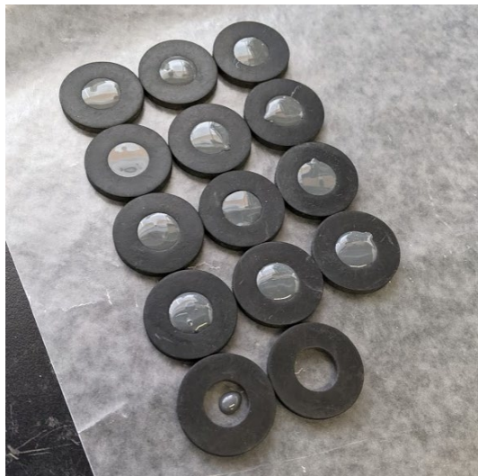
Fig. 32 Isolation Valve Wire Stoppers Being Molded
