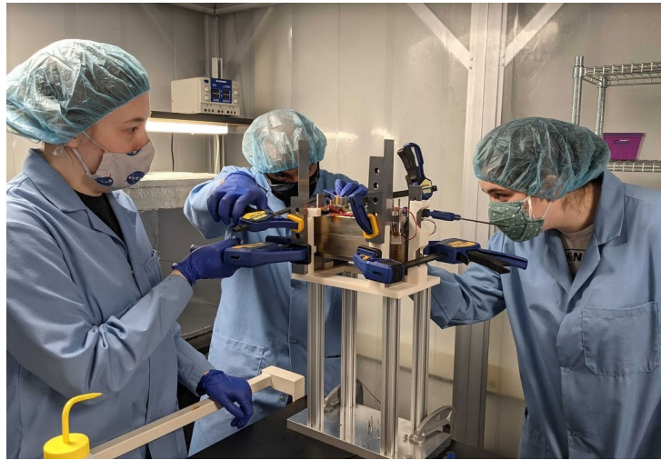
Fig. 23 Tank and Manifold Mounting Fixture
