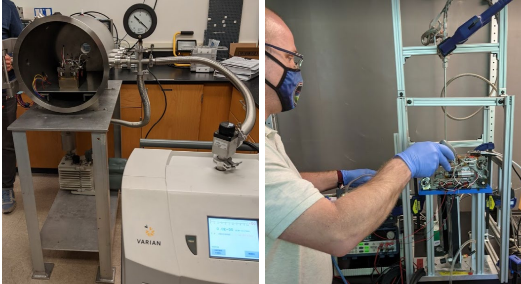
Fig. 29 Thruster Leak Test and Flow Test
