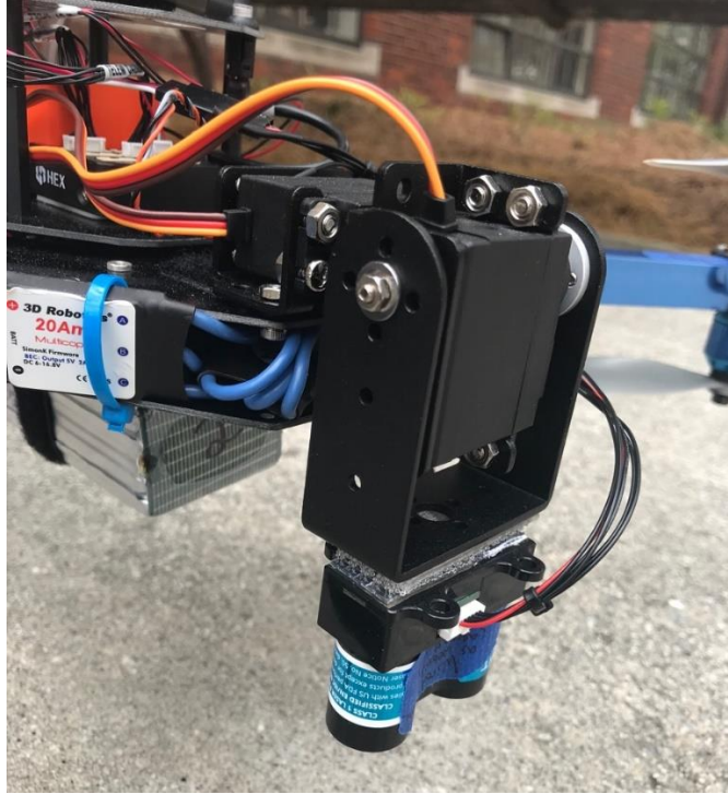
Figure 2. Lidar Sensor Mounted to Servo Gimbal
