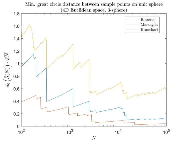
Fig. 29 Minimum great circle distance between points in samples of unit 3-sphere, d_0 , adjusted by \sqrt[3]{N_{\text{sequence}}} .
