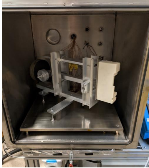
Fig. 16 Thrust stand set-up in GT SSDL TVAC chamber.
