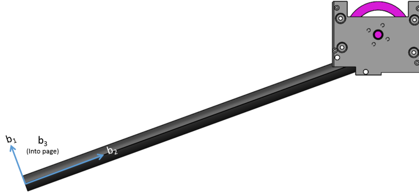
Figure 3.7: Boom fixed coordinate frame used to analyze the loads.
