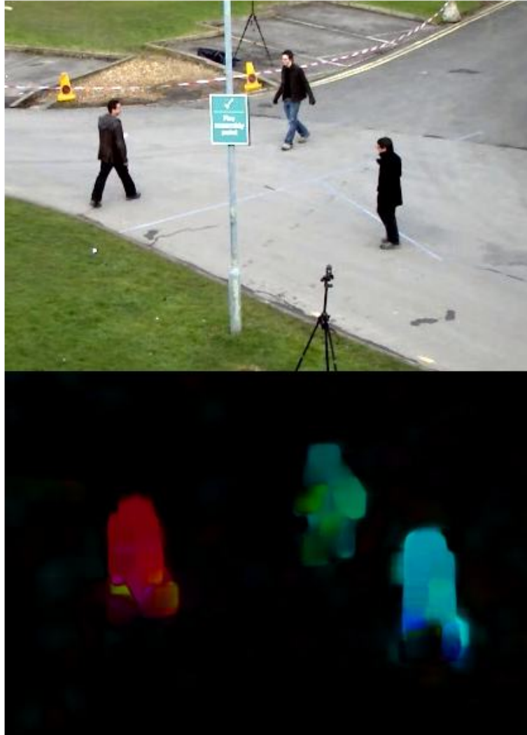
Figure 5.1: Dense optical flow using the Lucas-Kanade method [86]
