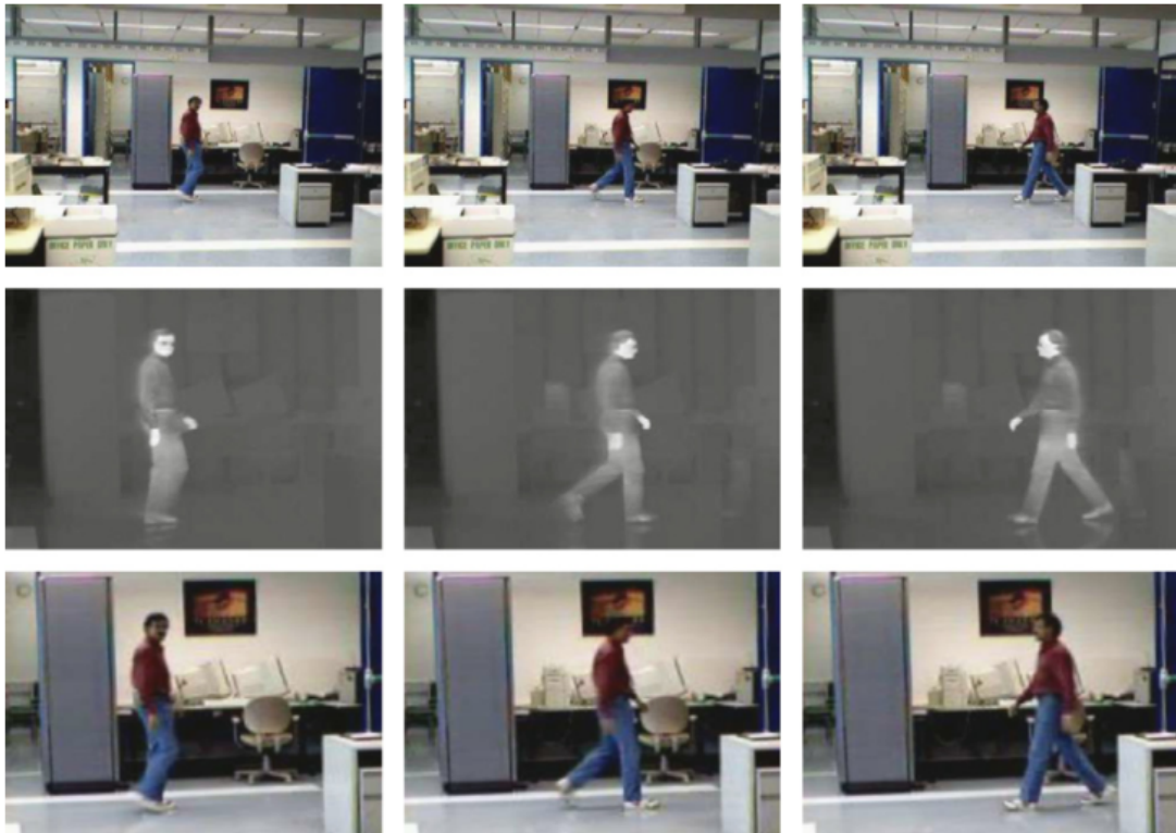
Figure 2.5: Color and thermal registration results from Han and Bhanu [34]: original color images (first row), original thermal images (second row), and transformed color images (third row)
