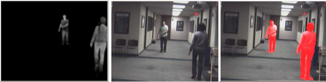
Figure 2.8: Infrared image (left), visible image (center), and human detection (right) [36]
