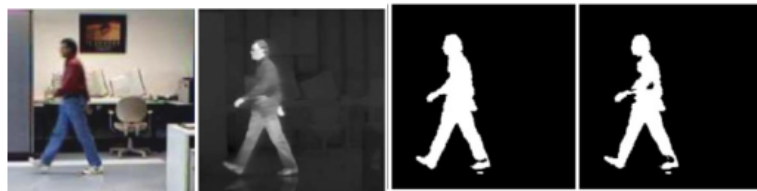
Figure 2.6: Transformed color image (first), thermal image (second), and silhouette fusion using two different methods (third and fourth) [34]
