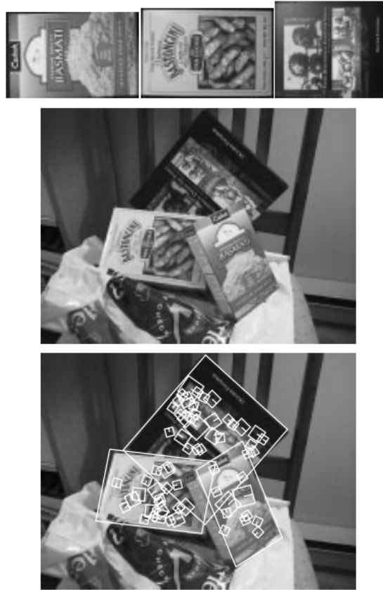
Figure 2.1: Model images of planar objects (top), test image (center), and recognition results showing model outlines and image keys used for matching (bottom) [12]
