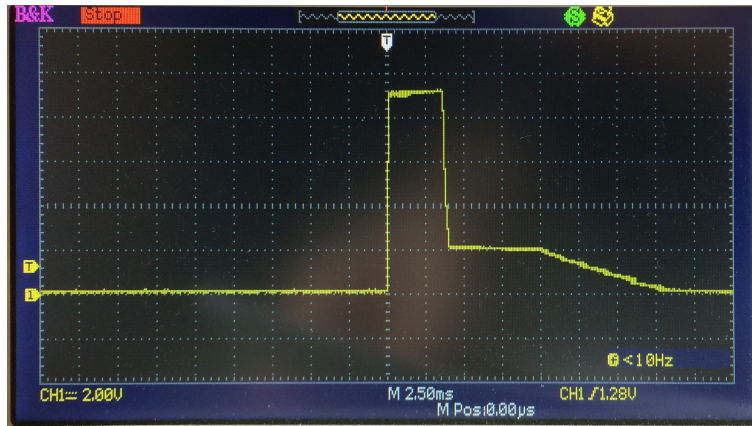
Figure 2.11: Oscilloscope capture of spike-hold voltage for a 10 millisecond pulse. Note that this was captured with no valve attached, so the voltage drains slowly when both switches are closed. With a valve attached, the final drop-off is sharp.
